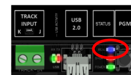
Blue LED Indication of polarity of the reversing loop track
